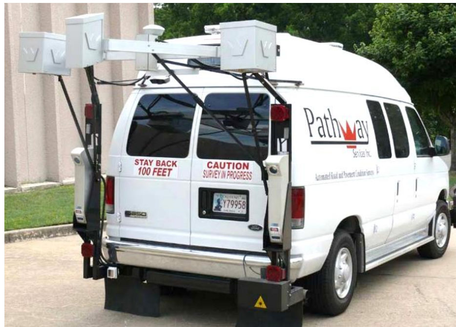
Figure 3: A "Pathrunner" Automated Data Collection Vehicle (Pathways) This is one of the van's that a previous data collection vendor used to collect pavement condition in Iowa from 2013-2017.
