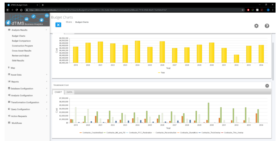
Figure 24: dTIMS BA Interface The dTIMS BA software is accessed through normal computer browsers and operates over cloud-based technology. Calculations are performed on remote servers, meaning any computer can use it, regardless of hardware capabilities!
